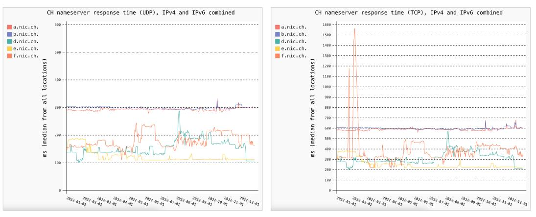
**UDP** response times *Combined response times of IPv4 and IPv6*
